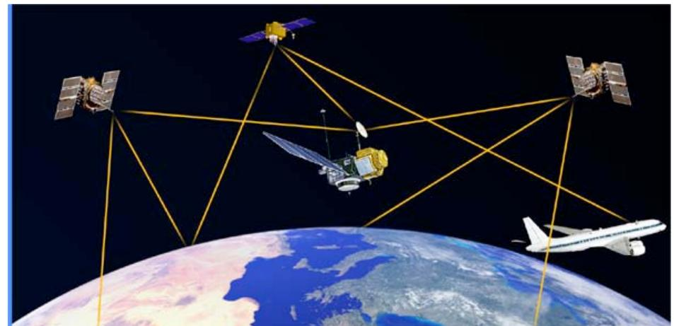
The NASA Global Differential GPS system is providing real-time global GPS performance/integrity monitoring services to operational GPS at the U.S. Air Force. With more than 70 real-time tracking sites, the GDGPS System tracks each GPS satellite by at least **9 sites**, and by **18 sites** on average, enabling robust, real-time GPS performance monitoring with **4 sec** to alarm.
